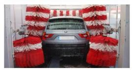
In installations from 12.5 meters, two additional vertical brushes can be installed to offer added value to the facility and higher wash quality.
