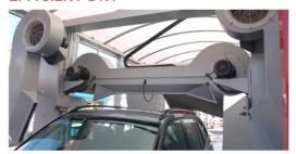
The dryer module is composed of 4 turbofans with 4 kW power each, working at low speed (1500 rpm) and with a high airflow rate for performance.
